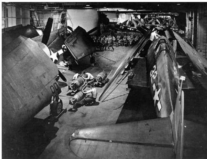
Figure 9 – Aircraft being prepared for a mission aboard USS Yorktown, the second of the Essex class carriers. The real superiority of U.S. Carriers was below the flight deck, with open hangars that had excellent working conditions and allowed aircraft engines to be warmed up, allowing the carriers to generate a much greater number of sorties than other navies' carriers
